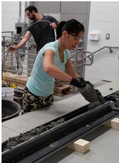
Figure 5: Placement of concrete
