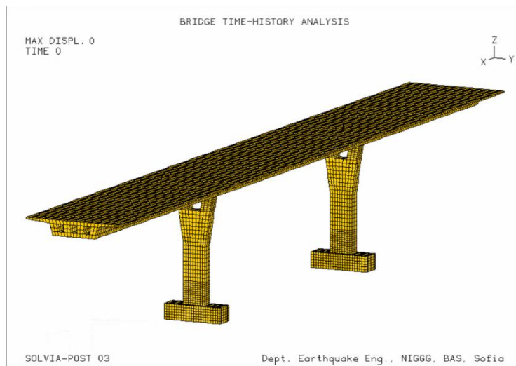
Fig 4. Three dimensional view of the finite element model.
